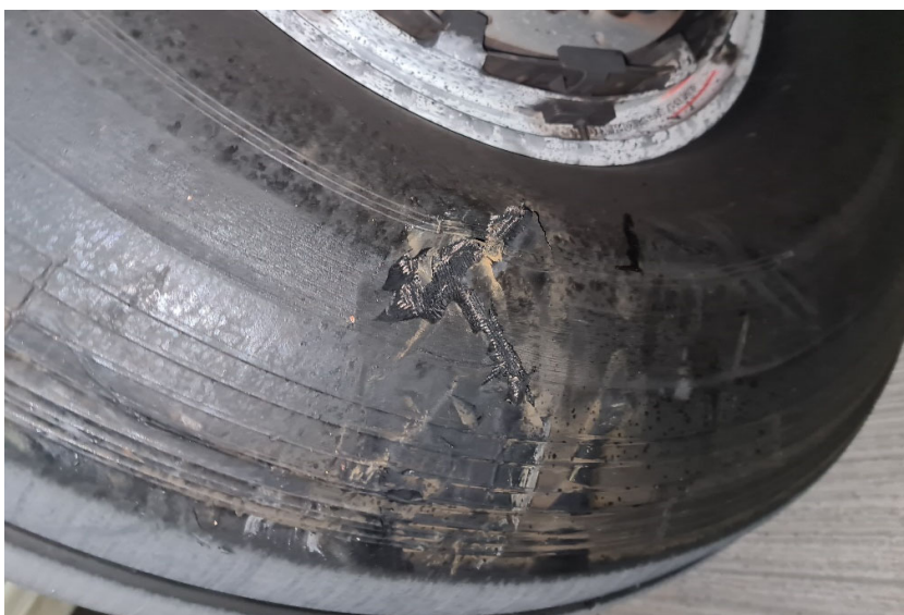
Figure 3 Damage to one of the landing gear tyres
